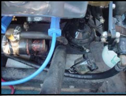
After the coupler was installed on the stock hose we routed it between the oil cooler and the fuel pump.
