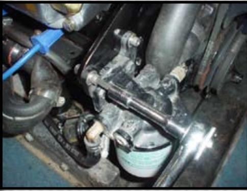
After the bracket installation on the front of the engine we re-install the water fuel separator with the supplied hardware.
