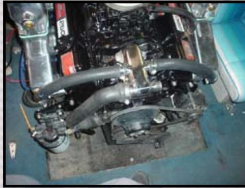
Using the supplied 1" water hoses we reconnected the 90 deg manifold fittings to the Sierra thermostat housing. Tighten all water connection clamps.
