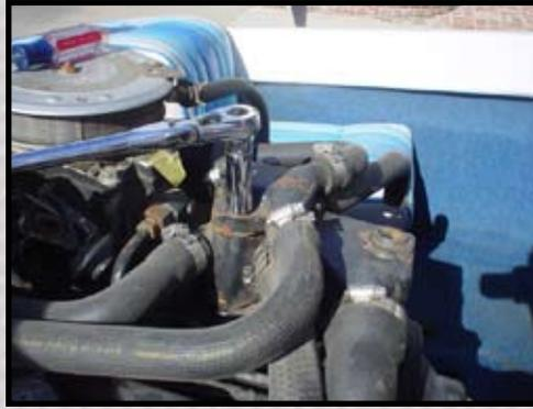
Remove stock thermostat housing, and stock cooling hoses.
