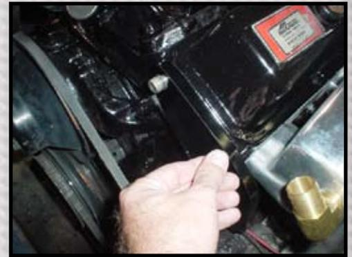
We then installed the new alternator bracket, with supplied stainless fasteners.
