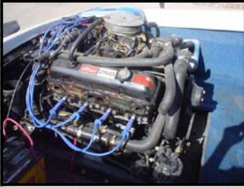
Remove stock exhaust manifolds, risers and stock rubber bellows from wishbone assembly. Remove old gasket material and prep for new install.
