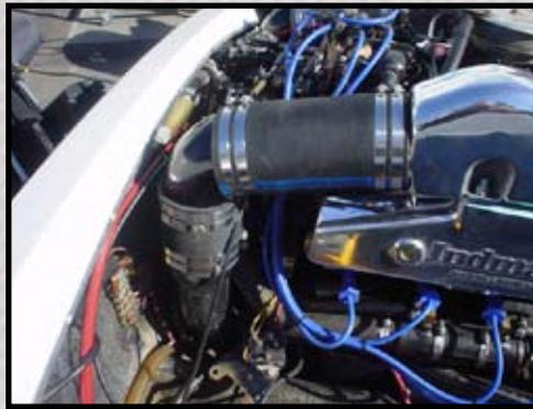
After manifold installation, we installed the new wishbone exhaust hose, 70 deg. elbows and manifold hoses. With the clamps left loose, we installed the riser gaskets and risers. After adjustments tighten all bolts and clamps.
