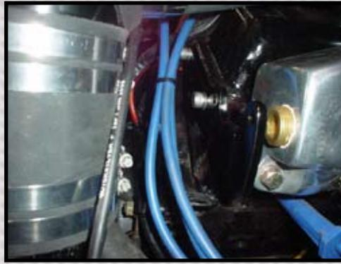
The new relay plate is installed on the starboard side rear of the head.
