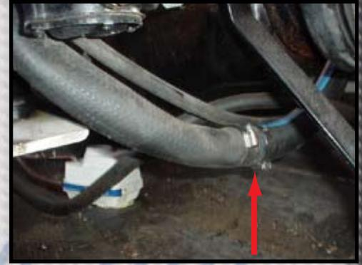
We then took the supplied 1 1/4" water hose, and attached it to the hose coupler. This extended piece of hose will now enable us to re-route the 1 1/4" hose to the thermostat housing.
