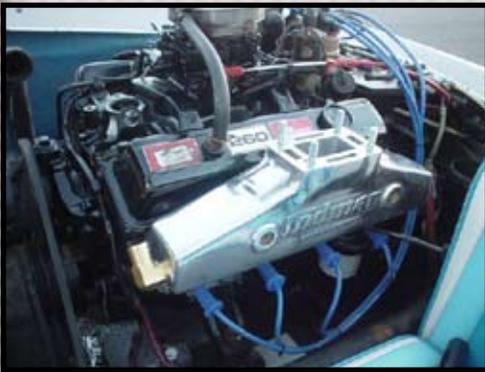
Before manifold installation, we have installed all of the required brass fittings and riser studs. Note: 90 deg. fittings are installed in the front of the manifolds and the plugs in the rear.
