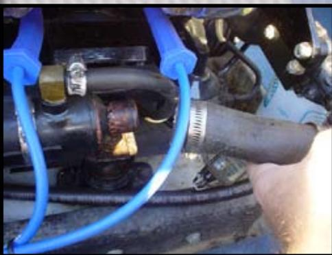
After the clamp was loose we had to pry the hose away from the cooler. Note: Be sure not to damage the inlet in the process.
