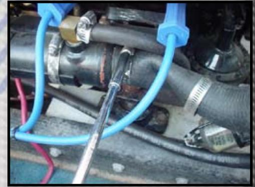
Next we removed the 1/4" water hose from the oil cooler.
