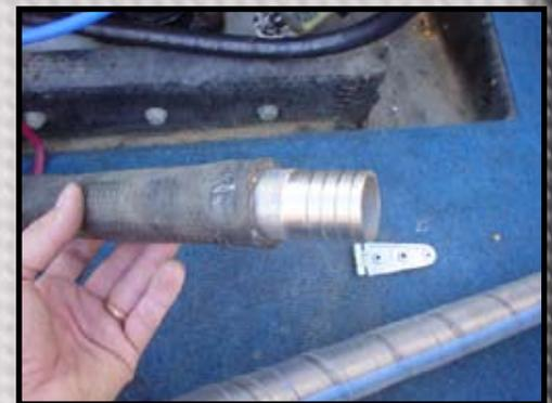
After the hose was cut, we installed the supplied coupler to the long straight side of the hose.
