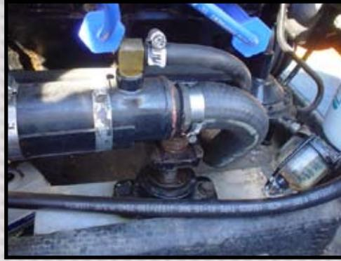
With the hose cut and routed properly, we re-attached it to the cooler.
