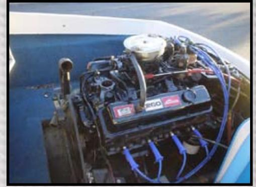
Clean thermostat area for new thermostat housing installation. Note: Main circulating hose stays intact with circulating water pump.
