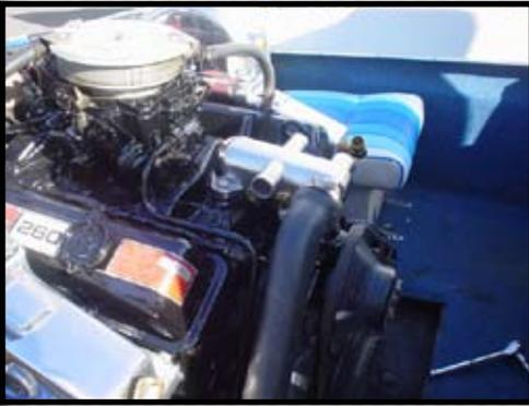
Install the new Sierra thermostat housing, and reconnect circulating water pump hose. Tighten the clamp.
