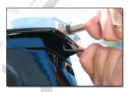
22. While applying pressure to the hose tighten the set screw on the underside of the billet cap.
