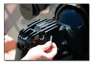
2. Once bolts are removed leave drive cap intact.
