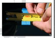
12. Measuring 3/4" from rear of cavitation plate mark first drill line.
