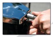
21. Push hose assembly into the shower cap to properly seat the o-ring.
