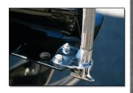
20. Install the remaining hardware to secure your pickup to the cav plate.
