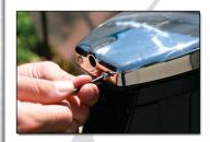
9. Using blue thread lock, install rear button head bolts.
