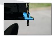
14. Drill left hole only using a 1/4" drill bit.
